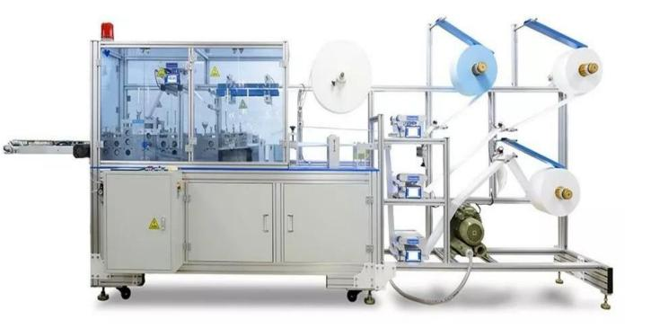
Differs to traditional earloop type mask making machine, this one-process mask forming machine gets rid of earloops and uses elastic bands, thus integrating the two separating process into one, which increases the production efficiency by 2.4 times, the masks produced are also much comfortable for long time wearing.
