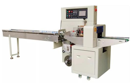
PLC controlled packing system, easy to set up, featured in servo motor film driving system, precise positioning, and solid sealing.
